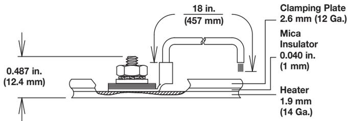
To install, mount the heater to the surface being heated and assemble mounting hardware. Standard measurements of assembly hardware are illustrated in the *Termination Assembly* drawing above. Please refer to the *Installation and Maintenance Manual (316-42-32-1)* supplied with the heater for mounting instructions.
