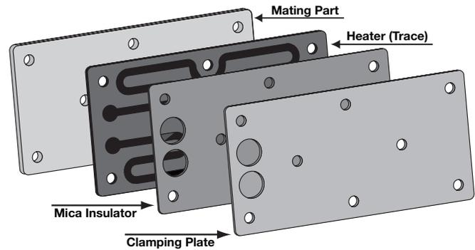
Thick film conduction heaters, designed for clamp-on applications, are supplied as a multi-part assembly: heater, mica insulator, clamping plate and mounting hardware.
