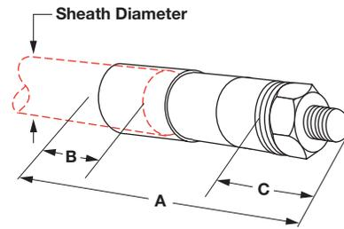
Ceramic-to-metal end-seals with threaded stud terminations provide an air-tight seal for continuous terminal temperatures up to 500°F (260°C). Watlow does not recommend this seal if terminations are exposed to temperatures exceeding 500°F (260°C).
