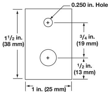
A 1 ½ in. (38 mm) x 1 in. (25 mm) wide x 16 gauge stainless steel bracket with one element hole and one mounting hole ½ in. (13 mm) from end.
