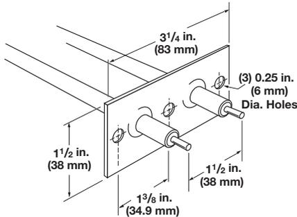
A 0.065 in. (1.7 mm) thick stainless steel bracket provides element mounting in non-pressurized applications. Attached to the heater sheath, these brackets are not suited for liquid-tight mountings. The bracket is located ½ in. (13 mm) from the sheath's end, unless otherwise specified.
