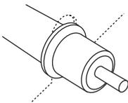
Stainless steel locator washers retain the heated area of the sheath in the work zone, while allowing for expansion and contraction during cycling.
