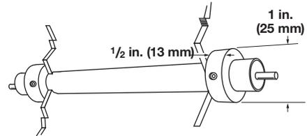
Plated steel mounting collars secure the heater sheath with set screws to serve as adjustable stops for through-the-wall mounting. Collars are shipped in bulk.
